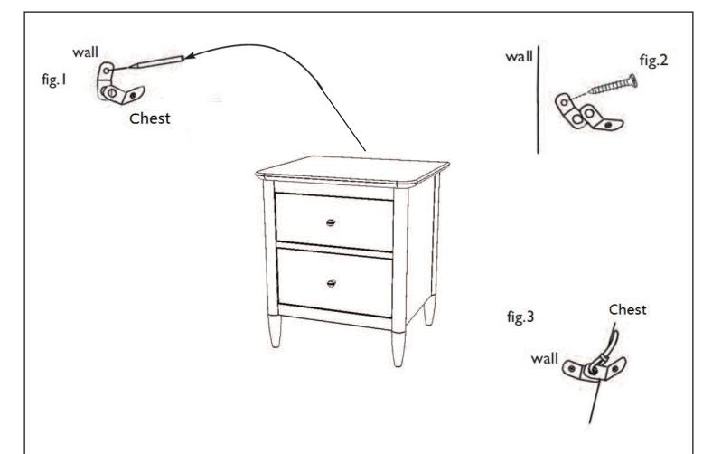
4. If the chest is not level on your floor use the wedges provided, and snap them off so that they do no Protrude out from the cabinet's legs, you can also snap them lengthways if desired.
